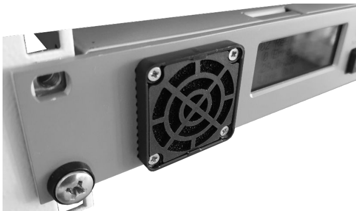
Figure 48. Mounted air filter on the fan opening of the device
